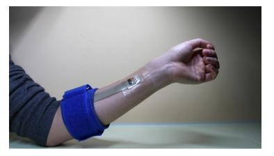
A research team from the Indian Institute of Technology, Bombay (IIT-B) has developed low-cost soft, flexible, and wearable sensors that can be used for diagnosis of pulse rate variability in humans.
