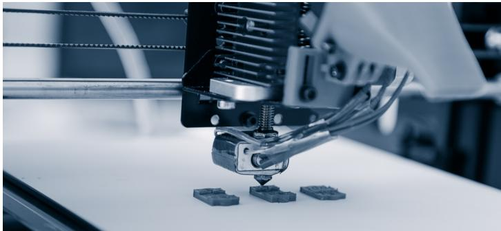
Manufacturing of cm-sized test specimens for material characterization according to ISO standards has now been achieved for the first time with a technology that allows 3D-printing a feature size of 200 nanometers.
